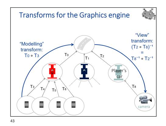
Transforms for the Graphics engine "Model-View" transform: T8<sup>-1</sup> • T2<sup>-1</sup> • T0 • T3 Τo **T**2 **T**1 Player's ł car T8 Тз T6 T4 T5 camera
