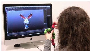
Tangible and Modular Input Device for Character Articulation Alec Jacobson, Daniele Panozzo, Oliver Glauser, Cedric Pradalier, Otmar Hilliges, Olga Sorkine- Hornung SIGGRAPH 2014
