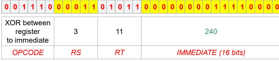
The diagram shows the 32-bit MIPS I-type instruction format. The first 6 bits are the OPCODE (001110). The next 5 bits are the RS field (00011). The next 5 bits are the RT field (01010). The remaining 16 bits are the IMMEDIATE field (00000000001111100000).
