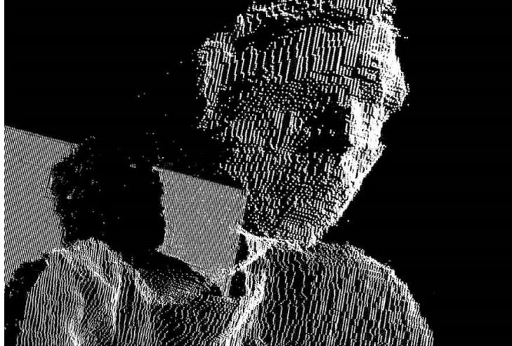
Output del kinect (una Depth camera)
