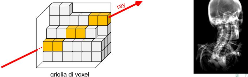
The diagram on the left shows a 3D grid of voxels. A red arrow labeled 'ray' enters from the bottom left and passes through several yellow-highlighted voxels. Below the grid is the text 'griglia di voxel'. To the right is a grayscale X-ray image of a human skull and neck, showing the internal structure. A small circular logo is visible in the bottom right corner of the slide.
