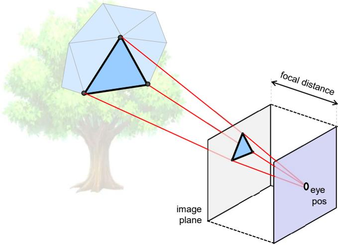
A diagram illustrating the rasterization process. A 3D scene with a tree and a blue triangle is shown. Red lines represent projection rays originating from an 'eye pos' (eye position) and passing through the triangle to an 'image plane'. The distance between the eye position and the image plane is labeled 'focal distance'. A small blue triangle is shown on the image plane, representing the projected 2D image of the 3D triangle.
